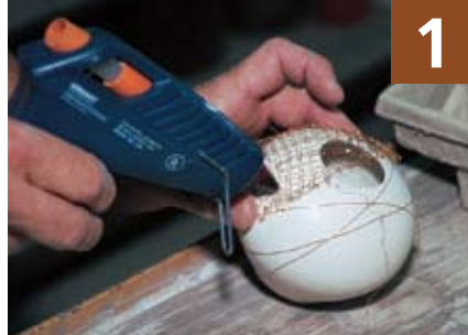
1 Copper mesh can be held in place with hot glue.
