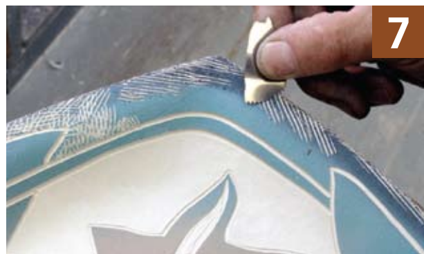
7 Cross-hatching is done with a serrated tool.
