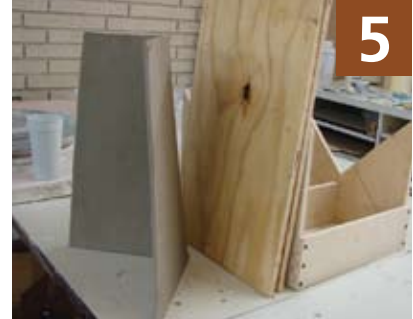
Two joined slabs stand after coming out of the jig.
