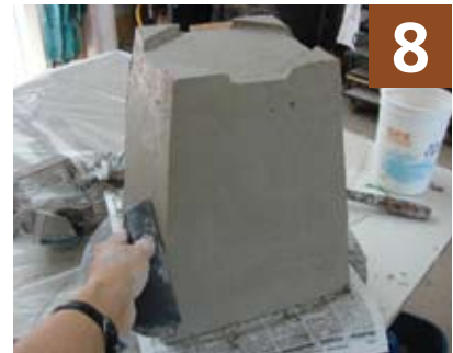
Refine edges with a Surform tool.
