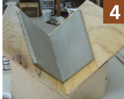
Butted slabs with 45° angles placed in jig.
