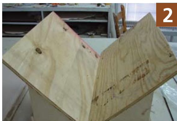
Two plywood boards complete the jig.
