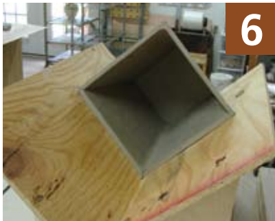
All four sides and the bottom are joined in the jig.
