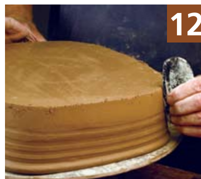
Smooth the slab and wall transition using a rubber rib.
