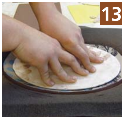
13 Use even pressure and press mold into clay.
