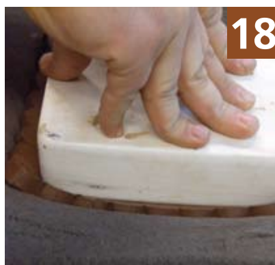
18 Press slab into foam.
