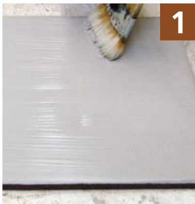
1 Prepare a slab and coat with slip.
