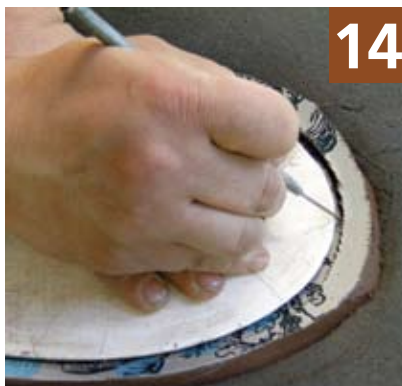
14 Hold mold down and trim remaining excess.
